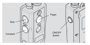
The transmitter for the **dogtra** 1900NCP Field Star single dog unit has four buttons (one on the face of the transmitter, two on the left side and one on the right side).
